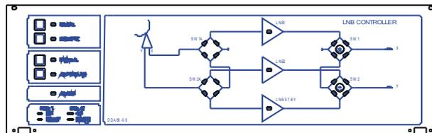
The DDA86-08 and DDA86-09 are versatile redundancy switches, intended for powering and protecting LNAs, LNBs and similar equipment. They have similar features, the main difference being that the DDA86-08 supports two LNA/LNBs in a 1+1 redundant configuration, while the DDA86-09 supports three LNA/LNBs in a 1+2 configuration.
