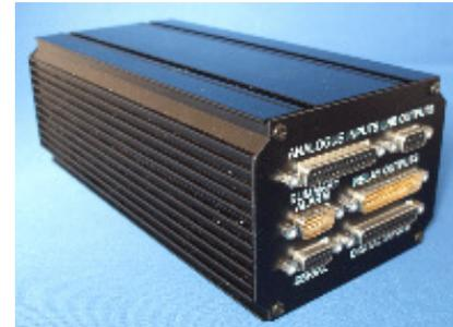
The DDA258 is a general purpose I/O unit for satellite ground station applications. It has been designed to transmit all heat to the outer casing, to simplify mounting in applications where air flow is limited.
